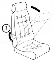
To tilt seat forward, turn knob (1) clockwise, push seat forward (right front seat only).
