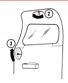
To open cabin door, twist upper door latch (2) forward lift the lower latch (3) up. Push door open.
